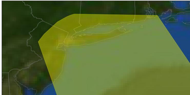
Figure 2-1: An example coverage map, with the coverage area in yellow. The station depicted here is WNYC-AM in New York City during the day. (AM radio stations can be received from much greater distances at night.) Only Radio-Locator's "distant coverage" area, the 50 decibel-microvolt signal strength contour, is shown.
